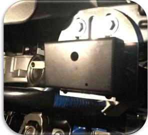
Plug in the lock and fix it with the provided M3 screws.
