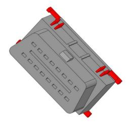
remove the plastic lugs marked red (e.g. witch a sharp knife)
