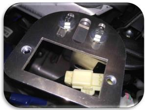
Place the retaining frame on the original OBD position and screw it to the base plate. Plug the OBD socket through the opening.
