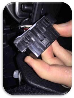
Remove OBD-Socket and remove the plastic lugs marked red (as shown on page 2)
