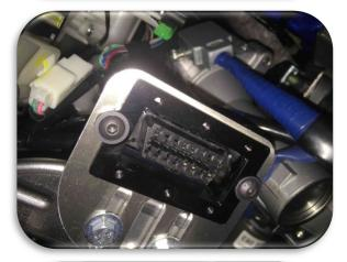
Bring OBD socket together with OBD-Saver lower part and screw into holding frame.
